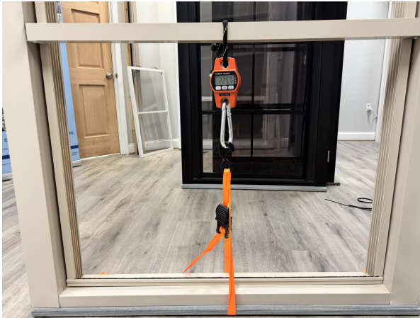
Fig. A.4.1-a: Downward load via crane scale
