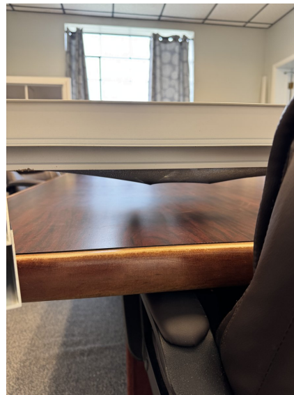
Fig. A.4.3-b: Deflection, no failure
