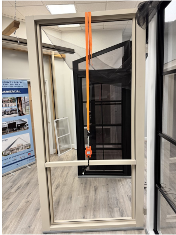
Fig. A.4.2-a: Upward load configuration
