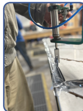
PNEUMATICALLY PRESSED INTO EXTRUSION @100PSI
